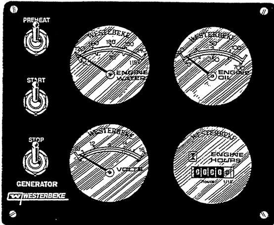
**PREHEAT:** The PREHEAT toggle serves two purposes: preheating the engine for easy starting and bypassing the engine oil pressure switch. The PREHEAT function closes the K2 relay, as well as supplies current to the fuel solenoid pull coil.
